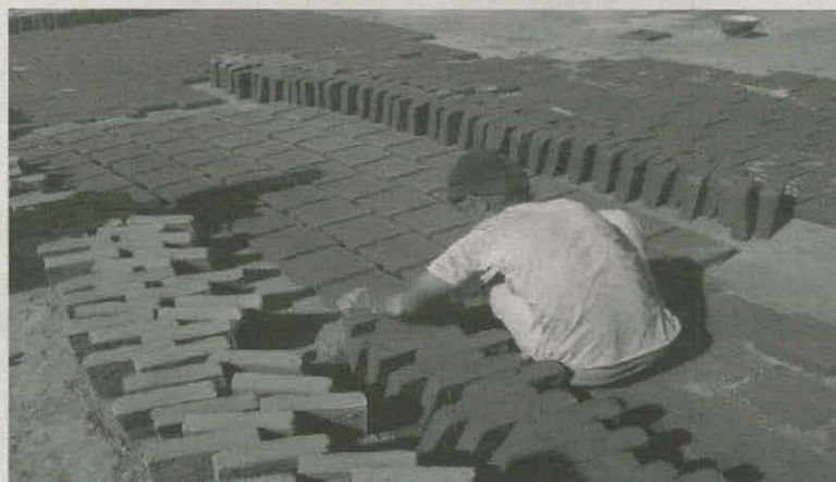
Figure 3– A mason making bricks using traditional techniques and materials in the Citadel.
