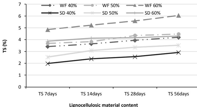
**Fig. 2.** Thickness swelling of wood/polymer composite manufactured with wood flour and sanding dust (WF=wood flour; SD=sanding dust).
