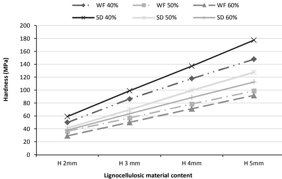
Fig. 5. Hardness of wood/polymer composite manufactured with wood flour and sanding dust (WF=wood flour; SD=sanding dust).
