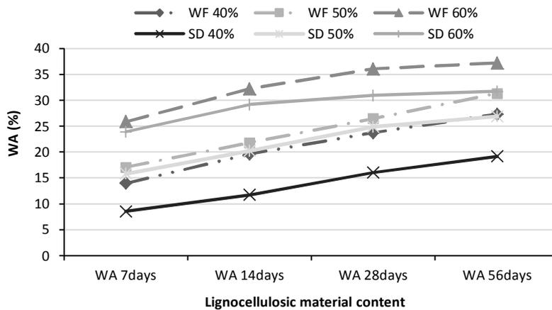
**Fig. 1.** Water absorption of wood/polymer composite manufactured with wood flour and sanding dust (WF=wood flour; SD=sanding dust).
