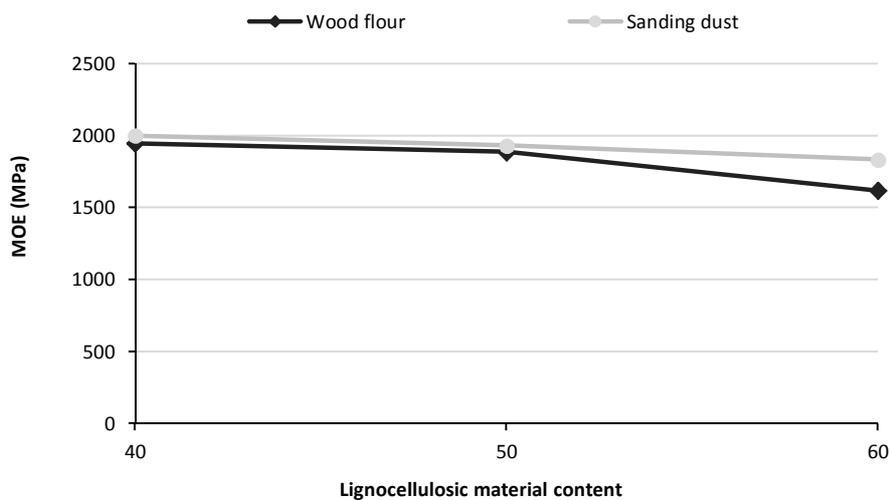
Fig. 4. Modulus of elasticity of wood/polymer composite manufactured with wood flour and sanding dust.
