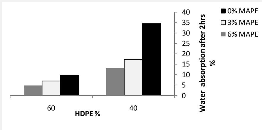
Figure 2. Interactive effect of HDPE% and MAPE% on water absorption after 2 hrs (density 0.8 g/cm<sup>3</sup>).
