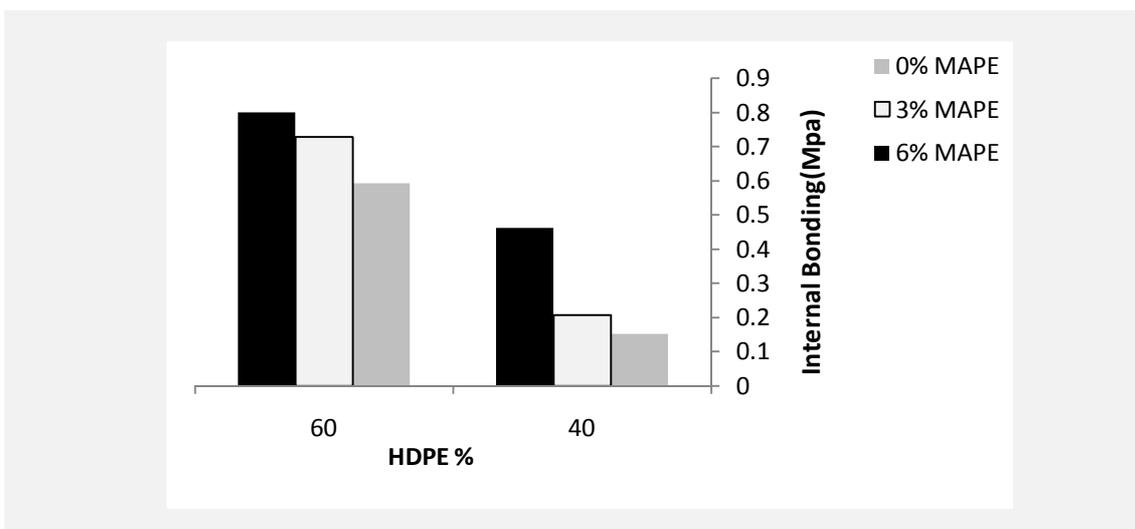
Figure 6. Interactive effect of HDPE% and MAPE% on internal bonding strength (density 0.8 g/cm<sup>3</sup>).
