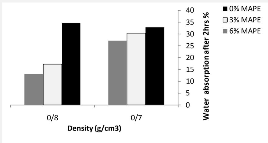
Figure 3. Interactive effect of density and MAPE% on water absorption after 2 hrs (HDPE 40%).
