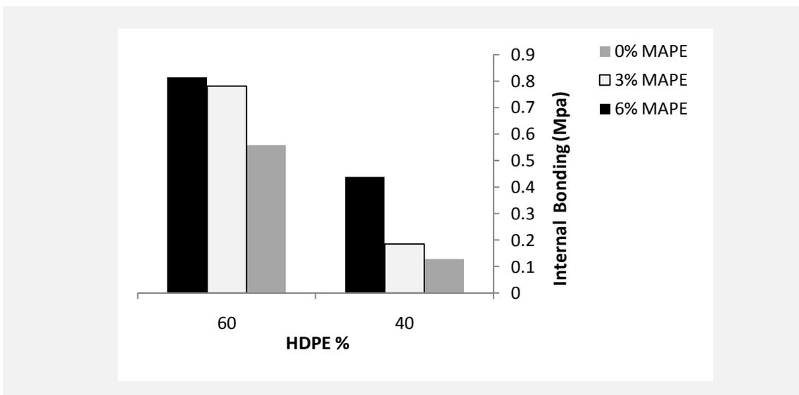
Figure 5. Interactive effect of HDPE% and MAPE% on internal bonding strength (density 0.7 g/cm<sup>3</sup>).
