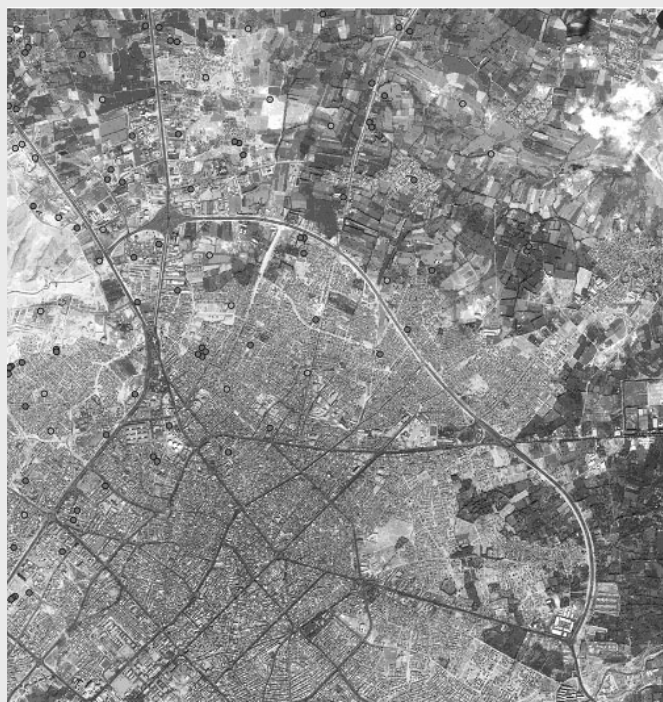
Figure1. The study area image and distribution of GCPs (dark points) and ICPs (light points).
