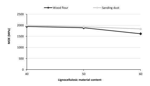
Fig. 4. Modulus of elasticity of wood/polymer composite manufactured with wood flour and sanding dust.
