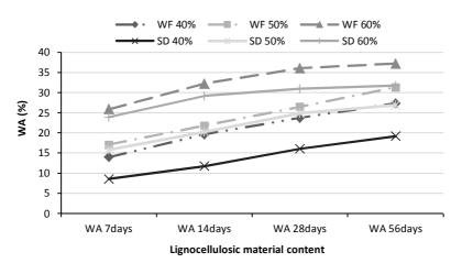
Fig. 1. Water absorption of wood/polymer composite manufactured with wood flour and sanding dust (WF=wood flour; SD=sanding dust).
