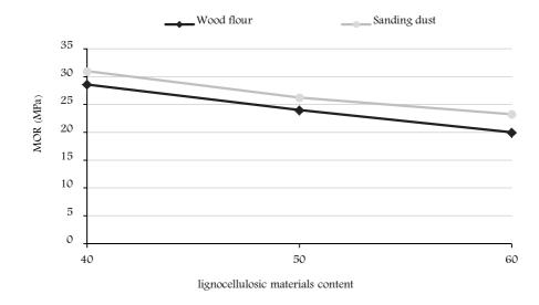
Fig. 3. Modulus of rupture of wood/polymer composite manufactured with wood flour and sanding dust.
