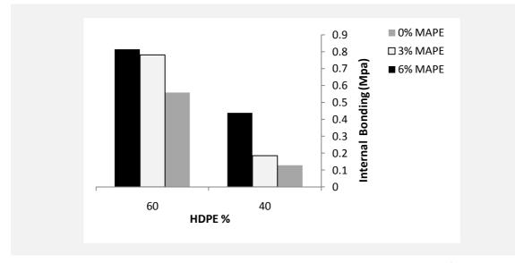
Figure 5. Interactive effect of HDPE% and MAPE% on internal bonding strengh (density 0.7 g/cm<sup>3</sup>).
