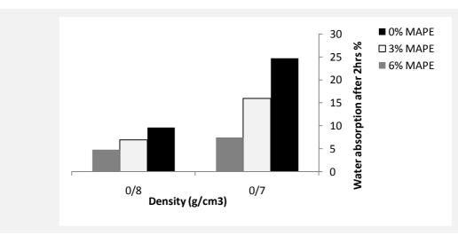
Figure 4. Interactive effect of density and MAPE% on water absorption after 2 hrs (HDPE 60%).
