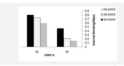
Figure 6. Interactive effect of HDPE% and MAPE% on internal bonding strengh (density 0.8 g/cm<sup>3</sup>).
