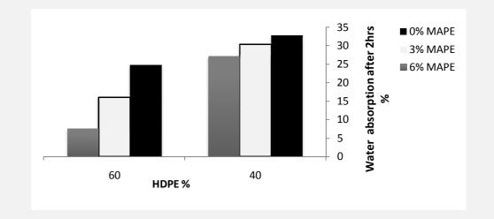
Figure 1. Interactive effect of HDPE% and MAPE% on water absorption after 2 hrs (density 0.7 g/cm<sup>3</sup>).
